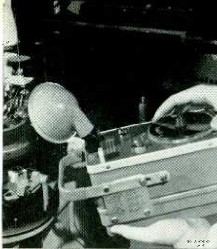
Strobotac used in hosiery knitting process to observe needle action.
