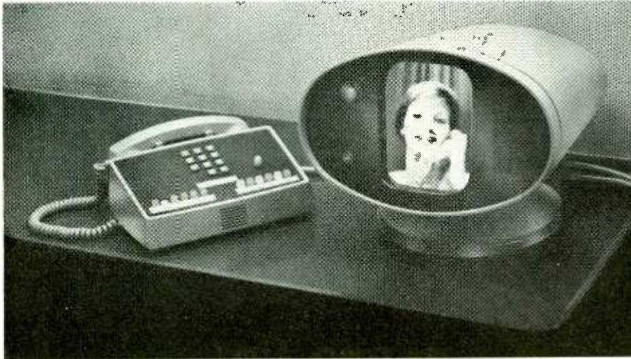
A person using AT&T's new Picturephone can push buttons to control whether he wants to be seen, see himself, see the other person, or nothing at all. Vidicon lens is small circle at upper left of screen. Speaker is behind grill to right. Control set uses no dial, but new "Touch-Tone" pushbutton calling system.
