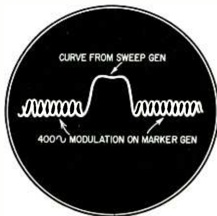
Fig. 8—Simple way to align traps is to use modulated marker signal at trap's frequency. When ripples along base line disappear, trap has removed marker.
